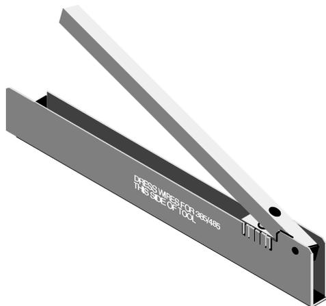
Figure 89 Modbus Plus Connector Installation Tool
