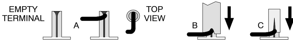
Figure 56 Wire Terminal Connection (Detail)
